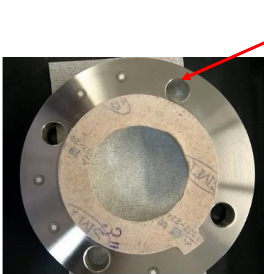
図3 Flange SUS316L: C \leq 0.030%
